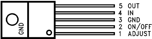
Figure 8. TO-220 5-Lead Power Package Front View
