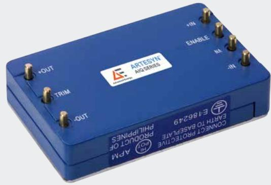
The AIQ02R series high voltage quarter-brick DC-DC converters accept a wide range 250 to 420 Vdc input and are designed for use with power factor correction (PFC) modules. Rated at 65 watts, the AIQ02R series can deliver full continuous power at operating baseplate temperatures from -40 to 100°C. The converters have a typical efficiency of 90% and produce a 28 Vdc output that can deliver up to 2.32 amps; the output voltage can be adjusted from 25.2 to 29.4 V with an external trim resistor.
