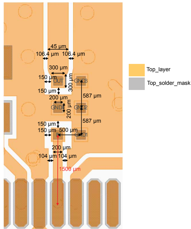
Figure 9. PCB land pattern recommendations
