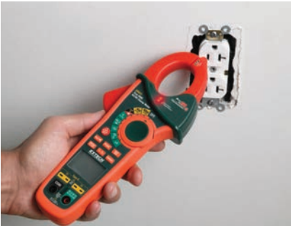
Non-Contact Voltage Detection.
