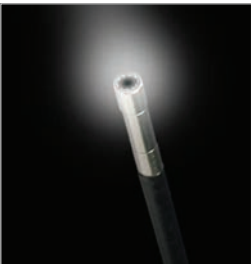
Camera Tip features built-in LED lights
