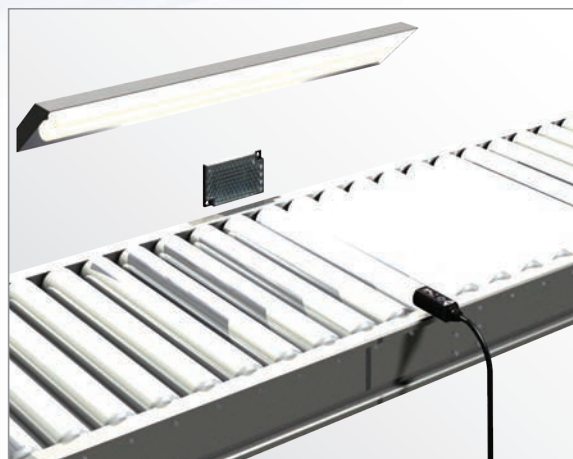
Pulse synchronisation for high ambient light immunity.
