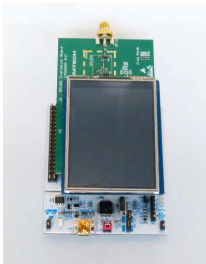
Figure 2: Touch screen, RF module and MBED board correctly assembled
