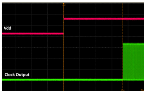
Figure 17. Startup Waveform vs. Vdd
