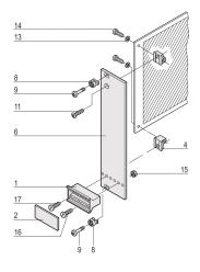
Plug-in unit, with static handle and the flat front panel. The grey handle is assembled on the front panel.
