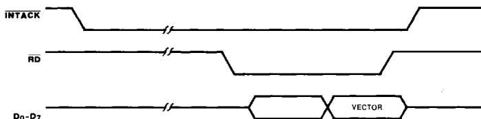
Figure 14. Interrupt Acknowledge Cycle Timing
