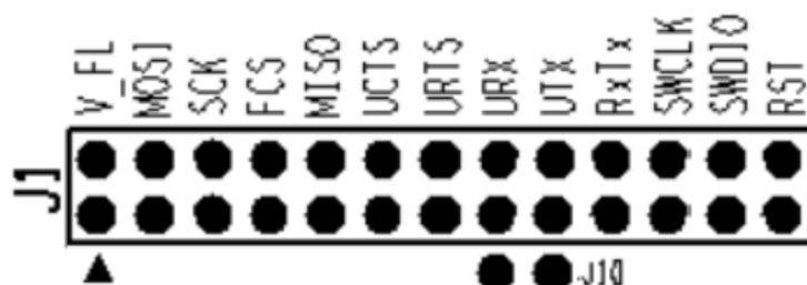
Figure 19: J1, Configuration Header on DA14531 PRO-MB
