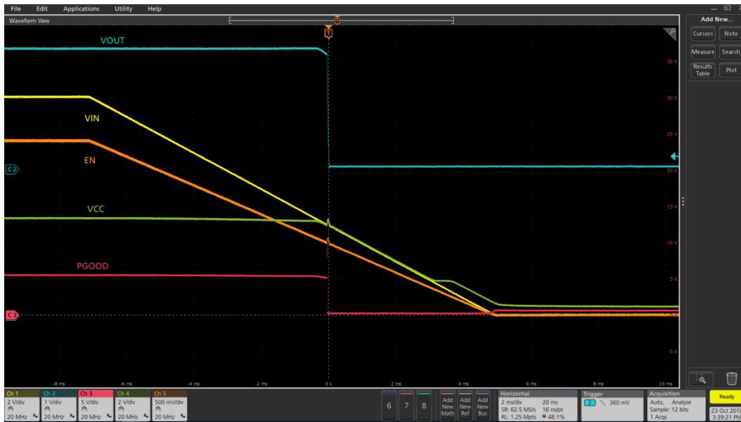
Figure 19 Shutdown with Enable de-assertion at 4A load (Ch1:PV IN , Ch2: V OUT , Ch3: PGood, Ch4:V CC , Ch5: Enable)
