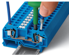
CAGE CLAMP® connection Inserting a conductor. With ferruled conductors, it is necessary to use a terminal block one size larger than the conductor's nominal cross-section.
