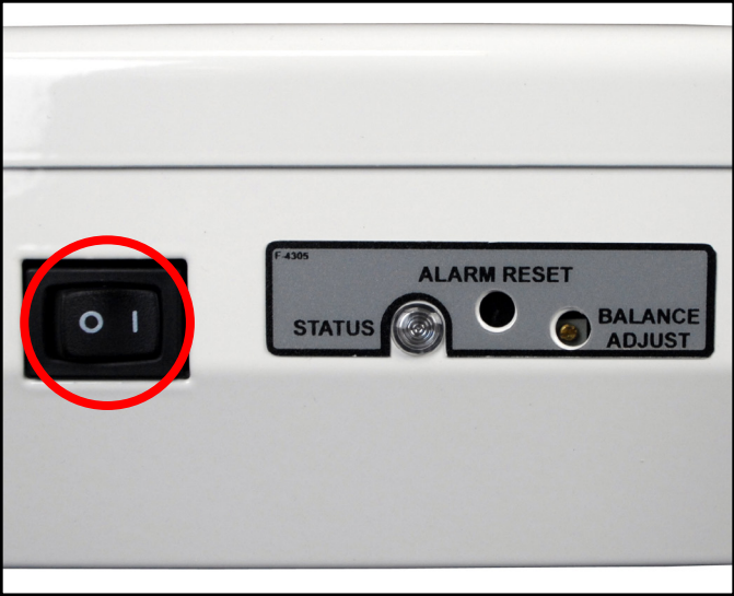
Figure 6. Light Switch (60467 and 60468 models only)
