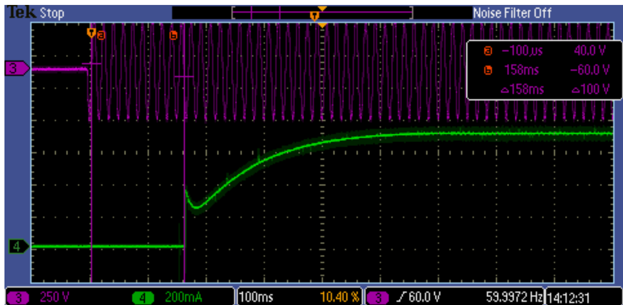
Figure 28. Start Up with AC Applied 277 V Maximum Load
