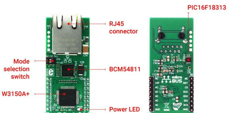
BroadR-Reach click has been designed to demonstrate and test 10 Mbps BroadR-Reach and 100 Mbps BroadR-Reach connectivity. However, the BCM54811 as a device is a triple-speed 10/100/1000BASE-T Gigabit Ethernet (GbE) transceiver. In addition to 10Mbps and 100Mbps BroadR-Reach connectivity, the transceiver can support 1000BASE-T, 100BASE-TX and 10BASE-T on standard Category 5 UTP cable. The 10BASE-T Ethernet can also run on standard categories 3, 4, and 5 UTP. The BCM54811 is designed to
