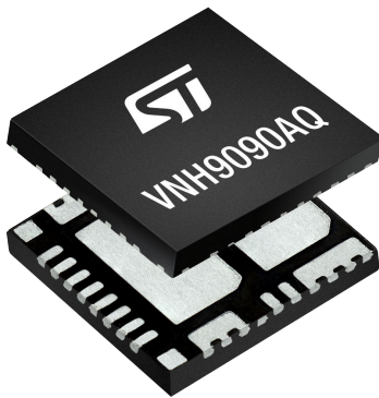
QFN 6x6 triple pad 26+2L
