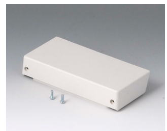
B4016417 Lid M closed, flat ABS (UL 94 HB) off-white RAL 9002 5.28"x2.44"x0.94"
