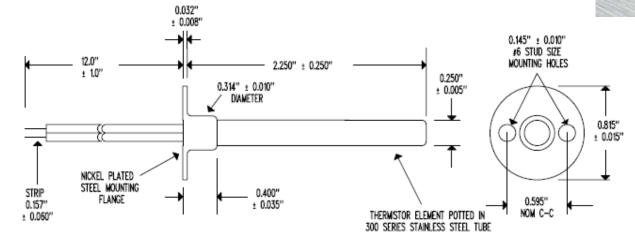
RESISTANCE \* +25°C = 10,000  $\Omega$  ± 1x resistance/temperature curve = "J" Temperature coefficient \* +25°C = -4.4x/°C nominal beta " $\beta$ " (0 to +50°C) = 3,892°K nominal maximum temperature rating = +105°C
