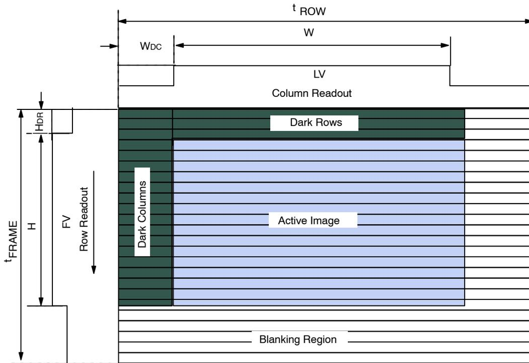
Figure 10. Frame Timing
