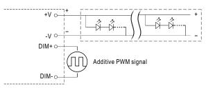
"DO NOT connect "DIM- to -V"
