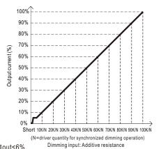
Note: 1. Min. dimming level is about 6% and the output current is not defined when 0%< Iout<6%.
