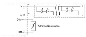
"DO NOT connect "DIM- to -V"
