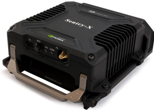
**Sentry-X is tested to meet MIL-STD-810G as well as DO160G for shock and vibration along with ingress protection of IP67.**
