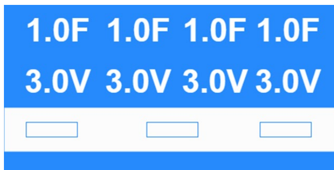
Example of the Markings of a 1.0F 3.0V capacitor
