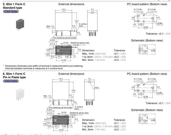
Dimensions (thickness and width) of terminal is measured before pre-soldering. Intervals between terminals is measured at A surface level.
