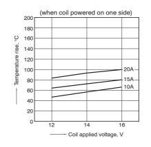
1.-(5) Coil temperature rise (at room temperature)
