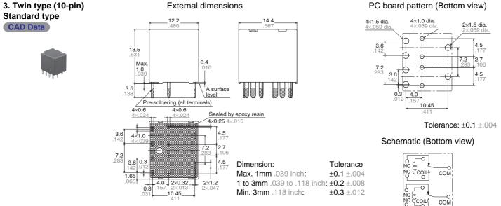
Dimensions (thickness and width) of terminal is measured before pre-soldering. Intervals between terminals is measured at A surface level.
