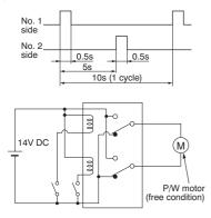
Load current waveform Inrush current: 25A, Steady current: 6A, Brake current: 13A
