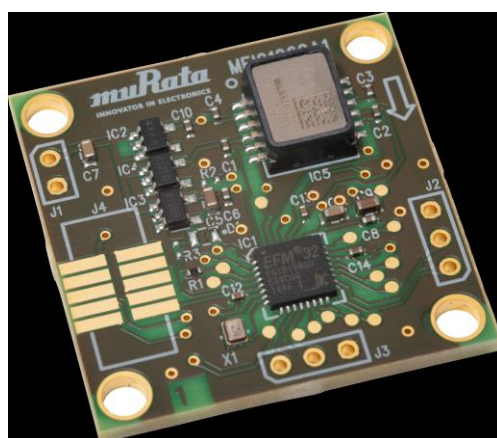
Figure 2 The BCGMCU-D01-PCB reference design sample
