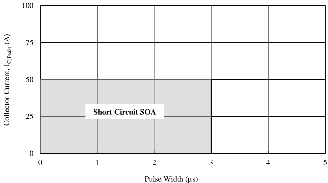
Figure 15-58. Short Circuit SOA: SIM6822MV, SIM6827MV
