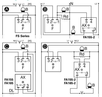
V = Voltage N = Neutral B = Beacon DL = Dummy Load for Constant Line Loading Rd =  $3.3 \text{ K}\Omega$  @ 5W for 120VAC;  $8.5 \text{ K}\Omega$  @ 5W for 230VAC F = Flasher (FS155-30T, FS155-30RF, FS165-30T)
