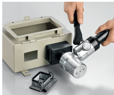
Automatic centre punching at the drill points when punching out holes for heavy-duty connectors.
