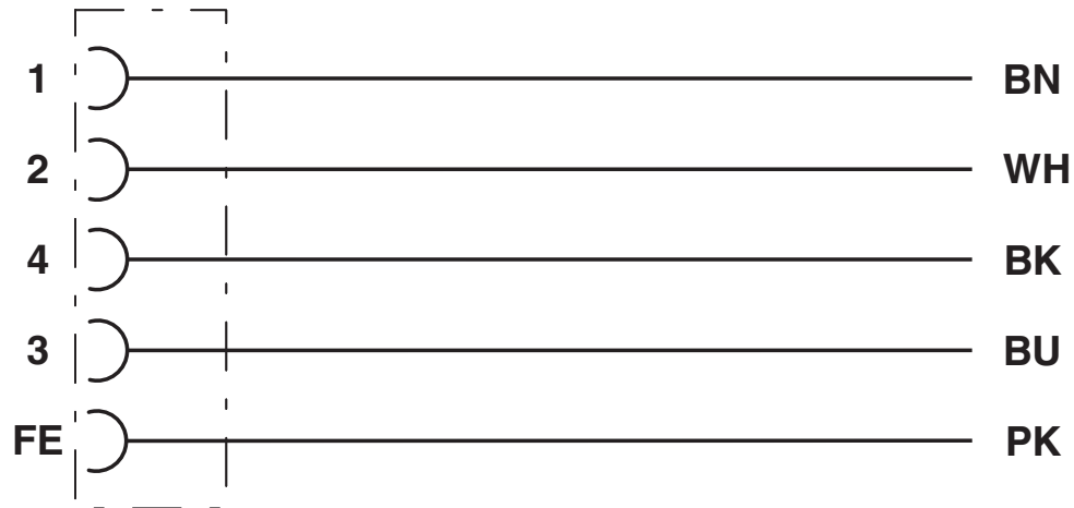
Contact assignment of the M12 socket
