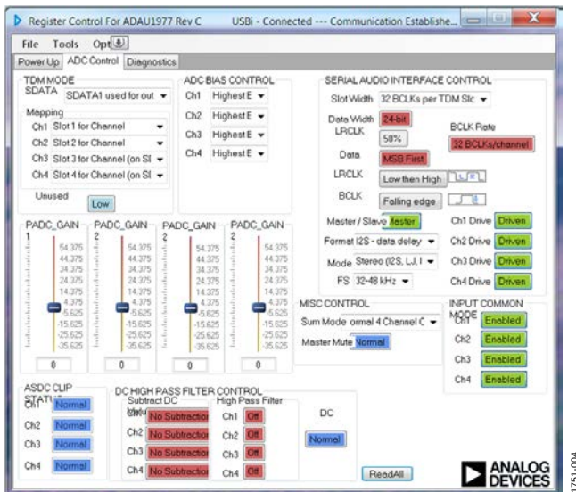
Figure 4. Register Control for the ADAU1977 GUI Page 2
