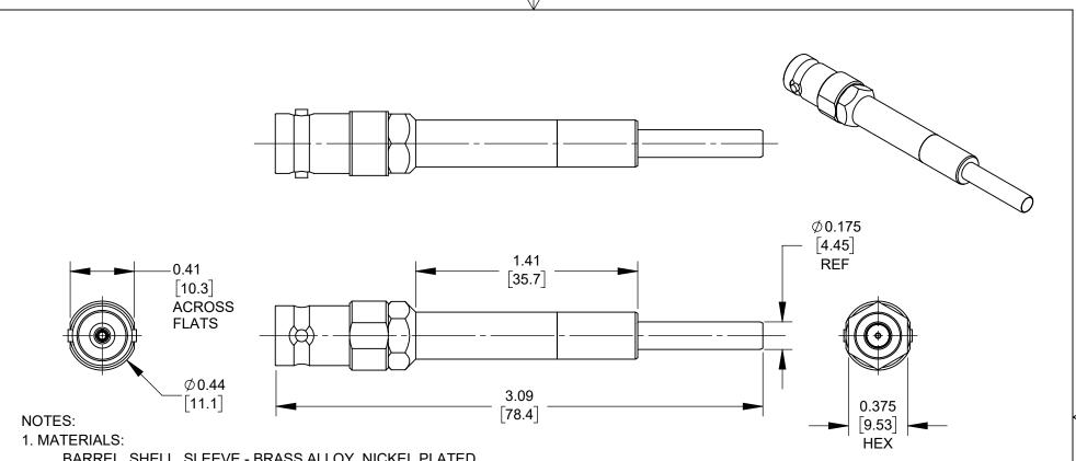
BARREL, SHELL, SLEEVE - BRASS ALLOY, NICKEL PLATED MICRO CONTACTS - BRASS ALLOY, GOLD PLATED BNC CONTACT - BERYLLIUM COPPER, GOLD PLATED INSULATORS - TEFLON
