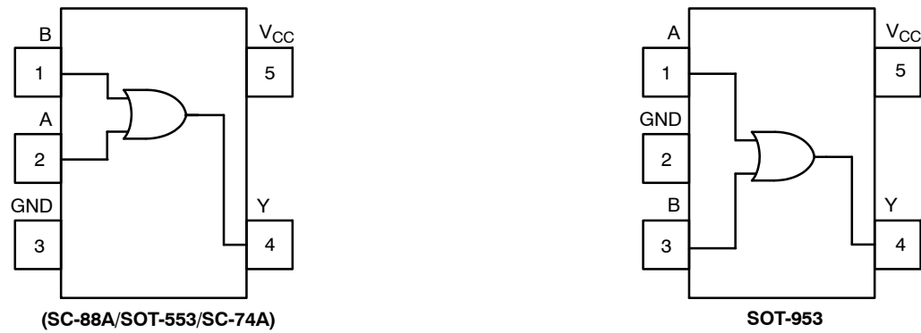
Figure 2. Pinout (Top View)
