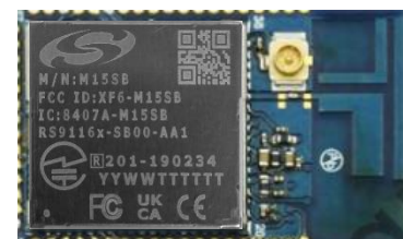
LGA Module (AA1) 27 mm x 16 mm
