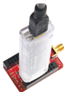
Fig-2: Programming and Debugging with CY8CKIT-002
