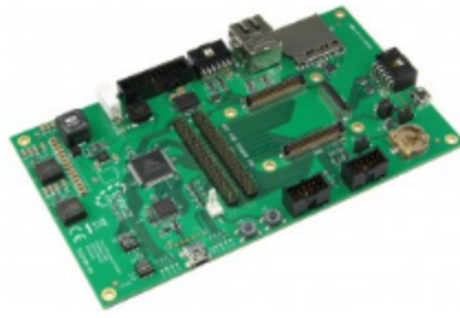
TE0705 - Simplified carrier board based upon TE0701
