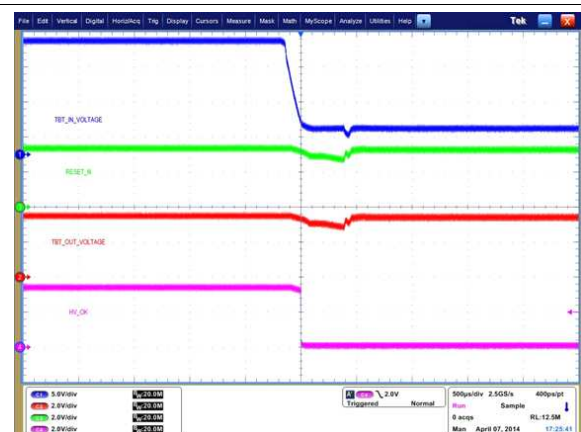
Figure 17. 3.3V to 0V Power Down With 50mA Load
