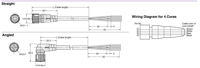
Note: Oil-resistant Polyurethane Cables (XS5F-D42 -- 80-P) and Spatter-resistant Cable (XS5F-D421- 80-SA) have black covers. Fireretardant, Robot cable (XS5F-D42 - 80-F) have warm gray covers.
