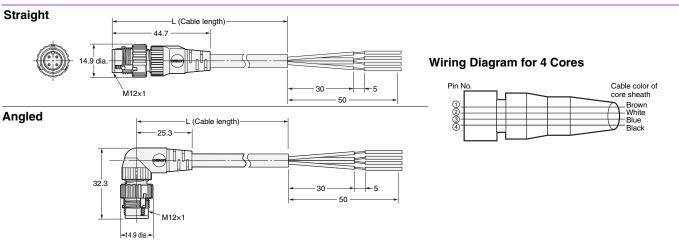
Note: Oil-resistant Polyurethane Cables (XS5H-D42 -- 80-P) and Spatter-resistant Cable (XS5H-D421- 80-SA) have black covers. Fire-retardant, Robot cable (XS5H-D42 -- 80-F) have warm gray covers.
