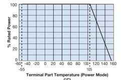
For resistors operated at an ambient temperature of 85°C or above, a power rating shall be derated in accordance with the above derating curve.
