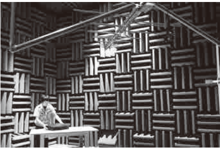
Acoustic radio wave anechoic chamber
