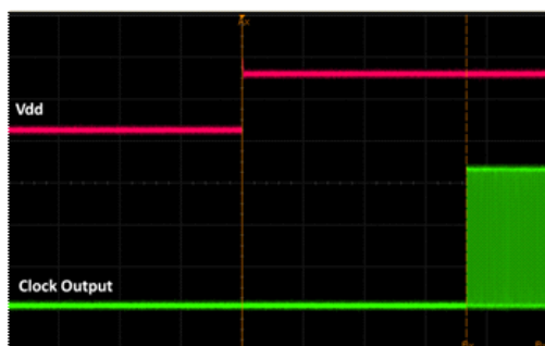
Figure 17. Startup Waveform vs. Vdd
