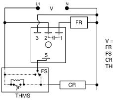
V = Voltage FR = Fan Relay FS = Fan Switch CR = Compressor Relay THMS = Wall Thermostat
