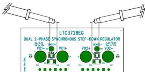
Figure 2. Output ripple measurement.
