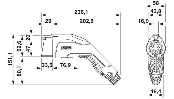
Make sure that the vehicle charging connector is placed in an appropriate charging connector holder, which ensures a minimum protection rating of IP24 in accordance with IEC 61851-1, for the entire time between charging. To create this charging connector holder, use the dimensions of the vehicle charging connector. Detailed dimensions can also be found in the Download area.
