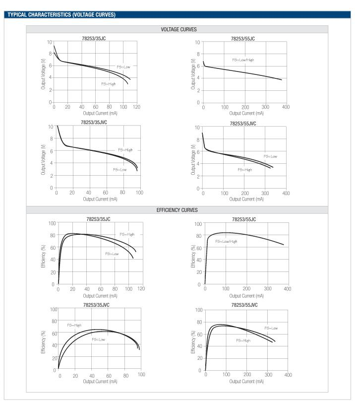
All curves are derived from testing with the Maxim MAX235 IC using the circuit shown in application note MPAN-03 (download at http://www.murata-ps.com/data/apnotes/mpan-03.pdf).
