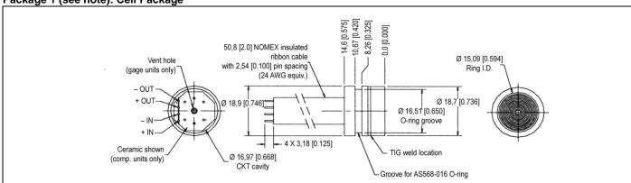
Note: Non-concentricity effects at the diaphragm weld area may cause runout of up to ±0.006 in between the upper and lower portions of the sensor body. (It is recommended to use a counter bore to mate with this device to allow for this non-concentricity).
