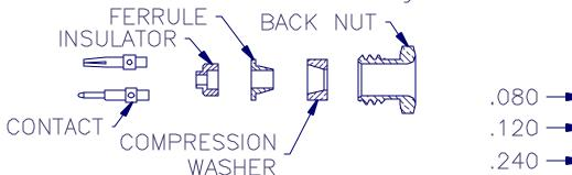
1. TRIM CABLE AS SHOWN. TIN END OF CENTER CONDUCTOR.
