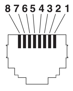
Connector pin assignment plug RJ45
