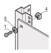
Cage nuts permit range of choice of nut and bolts sizes and easily replaced unlike pre-threaded holes. Cage nuts are easy to use on materials too thin or soft to be threaded.
