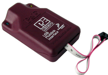
Figure 10-1: P&E's USB Multilink (USB-ML-12 shown)
