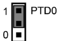
Figure 8-11: Accelerometer g-Select1 Jumper settings (J13)
