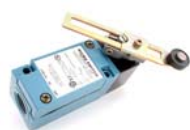
Series HDLS Non Plug-in: Side Rotary; 1NC 1NO SPDT Snap Action; 0.5 in - 14NPT conduit
