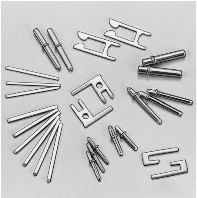
Various pins and wrap posts are available. The tips of the RT pins and the wrap posts are pyramid shaped to ensure smooth insertion into printed circuit boards. The RT pins are perfectly round since they are formed by drawing. The square wrap post is smooth on four sides but has sharp corners to ensure a secure and reliable wrapped connection.
